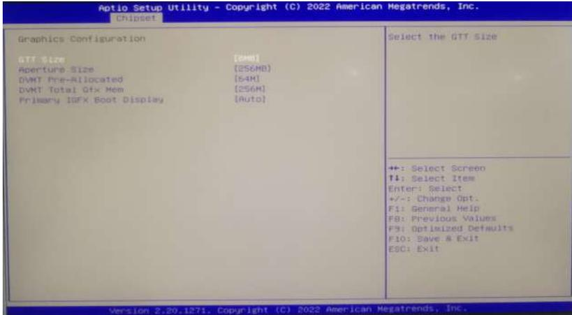
DVMT Pre-Allocated: Dynamically allocate the value of video memory.
