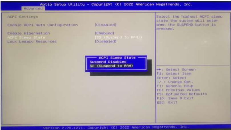
Enable ACPI Auto Configuration : This item is automatically configured for the ACPI, Allow (Enabled) or close (Disabled) BIOS ACPI automatic configuration, default is close (disabled).
