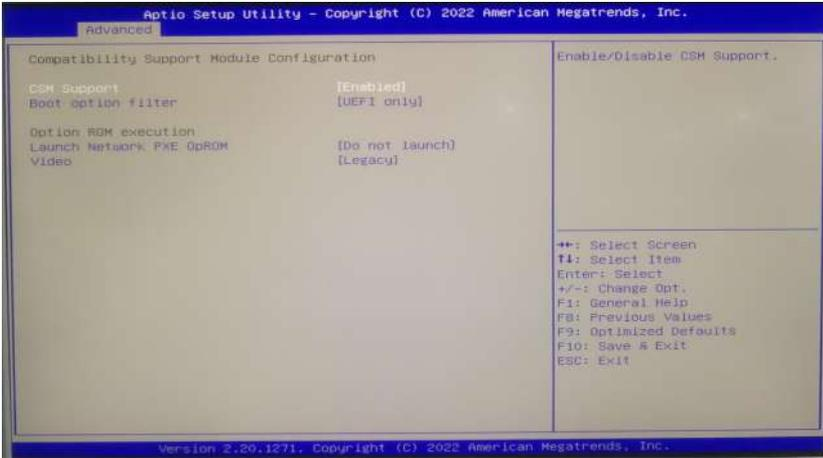
Launch Network PXE OpRom: set None-Disk boot; Do not launch: close None-disk boot; UEFI: set non-disk boot mode as UEFI; Legacy: set None-Disk boot as Legacy mode.
