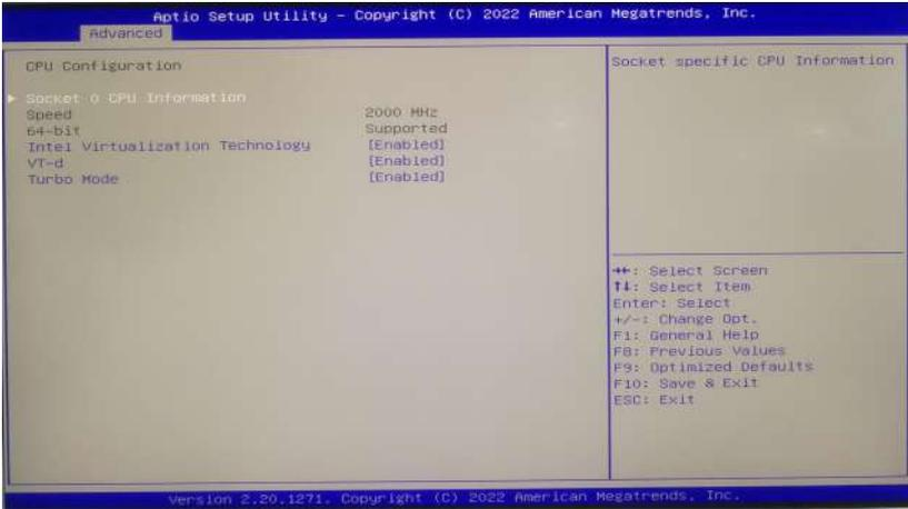
Read only items contain details of the CPU, including the CPU manufacturers, models, frequency, the first level cache size, the second level cache size and other information.
